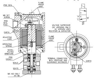
The pressurised media is retained within the valve assembly (pressure boundary) by the mechanical strength of all its metal parts, seats and seals. Degradation of any of these components will cause the valve to leak.
